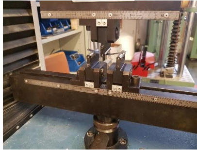
Fig.5. Bending test in three-point configuration
